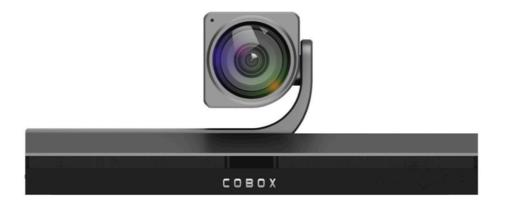
The X1 is a new generation of all-in-one multi-function terminal supporting H323/SIP, H264HP and H265 encoding. It uses 4K camera and built-in crystal high-definition microphone to bring you an extraordinary ultra-HD conference experience; Wi-Fi/4G wireless interconnection solution, The rapid deployment and use of conference rooms is the best choice for small and personal video conference construction.
